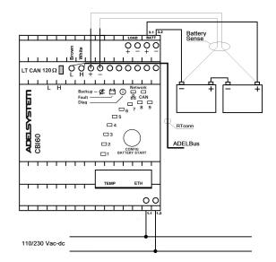
Connect two additional wires from the Battery Sense terminal of the device, to the Battery posts + and -; HR40004 provides the Voltage measured from the battery sense. The battery sense wires allow the battery voltage to be accurately measured without the influence of any possible ohmic drop due to charging/discharging currents in the battery power cables
