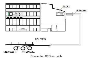
For the ADELBus connection, please connect the cable RTConn to AUX1 on the device as shown in the picture above and connect the other side of the cable to the CAN terminals L (Brown) and H (White) of the CBI60.
