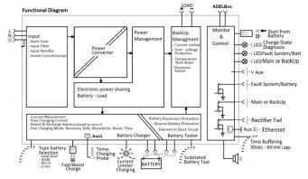
Input: Single-phase 115 - 230 - 277 Vac Output Selectable Load: 48Vdc 1.25A Output Battery charging:48 Vdc 1.25A Suited for the following battery types: Open Lead Acid, Sealed Lead Acid, lead Gel, Ni-Cd, Li-Ion Automatic diagnostic of battery status, Battery Life
