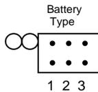
1. Sealed Lead (Charge): Trickle =2.25 Fast=2.40/cell
