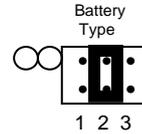
3. Gel Battery (Charge): Trickle =2.30 Fast=2.40/cell
