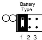
2. Sealed Lead (Charge): Trickle =2.27 Fast=2.40/cell
