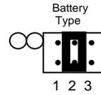
1. *Sealed Lead:* Fast=2.40V/cell      Trickle=2.25V/cell
