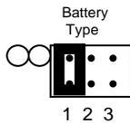
3. *Gel Battery:* Fast=2.40V/cell      Trickle=2.30V/cell
