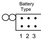
2. *Sealed Lead:* Fast=2.40V/cell      Trickle=2.27V/cell
