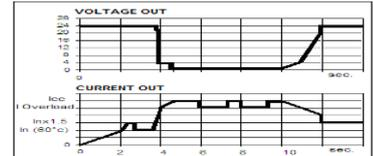
The output of the device is electrically protected against overload and short circuit. For the nominal output and nominal current at temperature condition, please see technical data. The device can supply at the nominal Current without switching off. As the overload increases, the output voltage is reduced until zero.
