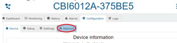
and the network page appears, showing the device configuration info: look at the “Enable DHCP” checkbox.
