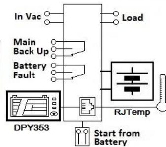
**Output Load:** power supply 24 Vdc; 10 A
